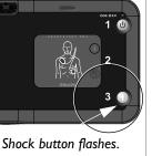
The Caution light stops flashing and stays on, and the orange Shock button starts flashing. The FRx tells you to press the flashing orange button. You must press the Shock button for a shock to be delivered. Before you press the button, make sure no one is touching the patient. When you press the Shock button, the FRx tells you that the shock has been delivered. Then the FRx tells you it is safe to touch the patient instructs you to begin CPR, and advise
